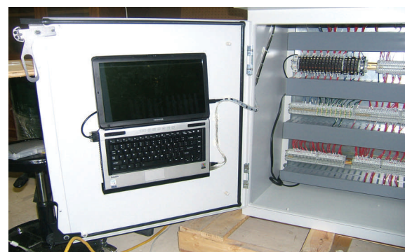
The XL BatchReports PC is an off-the-shelf laptop, allowing easy upgrade and maintenance.
